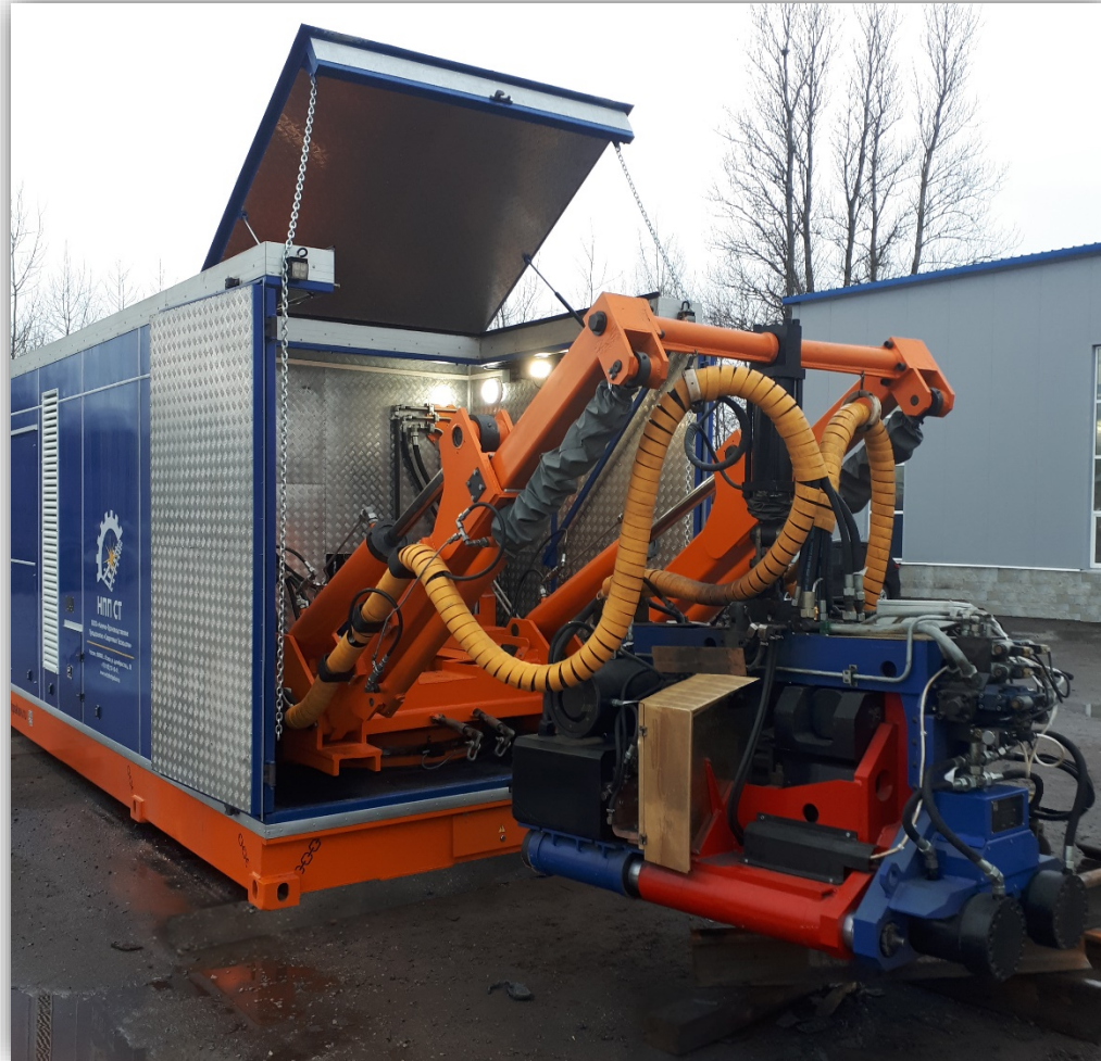
Suspended rail welding machine MSR-120.02 as part of the complex MRK-01ST
